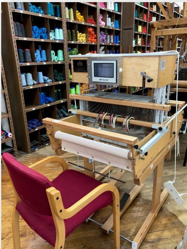
3 - One of only two looms which is semi-computerised and enables the user to sit down. It still requires someone to thread the loom with manual dexterity and ability to access the loom.
